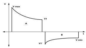
The waveform is adjusted to compensate for measured patient impedance as follows:
